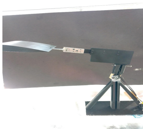
Figure 2. Connecting the wing model to the force system
