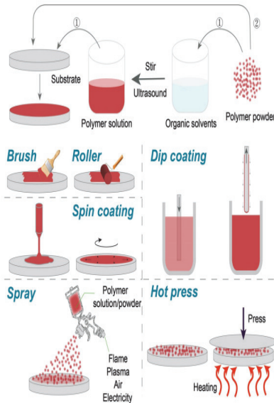
Figure 1. Various methods used in the preparation of polymer matrix composite coatings [16].
