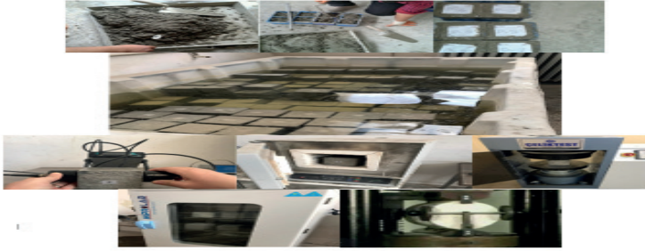
Figure 1. Natural fiber added lightweight concrete production scheme
