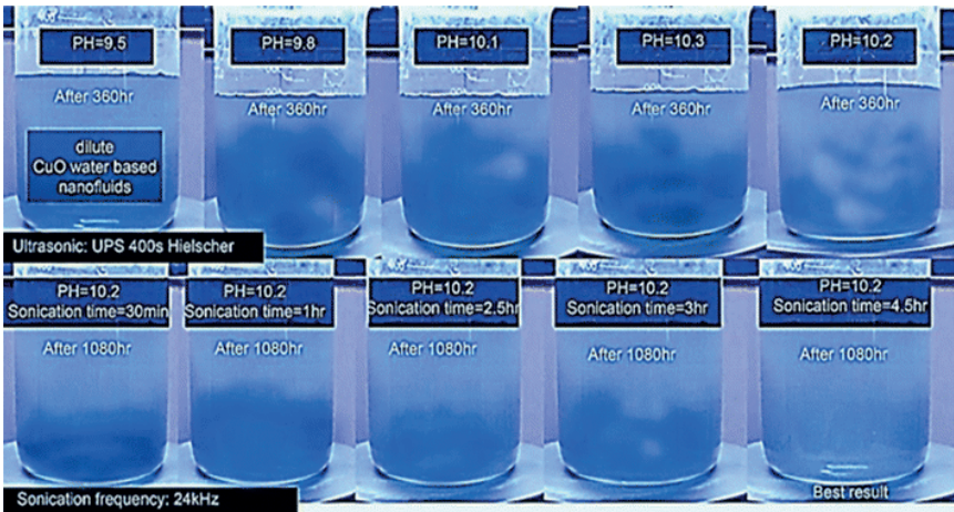
Fig.4. Effect of pH regulation on the stability of CuO/water nanofluids (Kamalgharibi et al. 2016).
