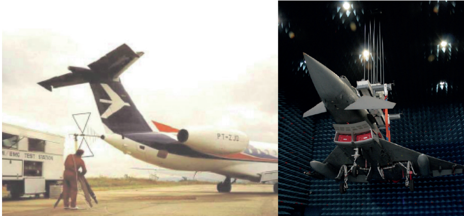
Figure 4. EMC testing of two airplanes in the open area and anechoic chamber
