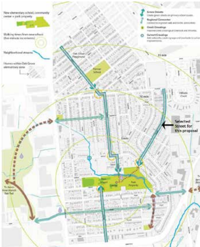
Figure 14. Bellemeade Green Street Project Plan
